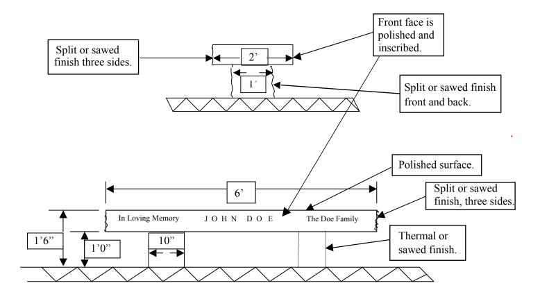
The stone will be granite. The bench will be 6 feet long by 2 feet wide. The top of the seat will be 1 foot by 6 inches from the ground. The top slab will be 6 inches thick and will be polished on the top and front surfaces. Inscriptions may be placed on the front surface only. The TSVC Deputy Director must approve all inscriptions before the bench is ordered.
